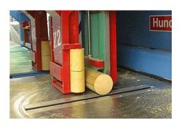
When processing a work piece lengthwise, e.g. slots and rabbets slipping between the positioning wagons and the work piece may occur. This would be indicated by an incorrect placement of the process step that follows the machining of the slot or rabbet. The SPCP automatically moves work processes that may experience slipping to the very end which means that no other steps will follow. Should there still be issues in this regard, try to influence the result by selecting
