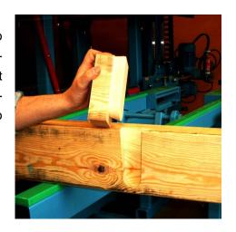
If the setting for the dovetail cutter is  $\rightarrow$  *machine data* (*d*)  $\rightarrow$  *operations*  $\rightarrow$  *Dove tail mortises on fence side*  $\rightarrow$  Yes there could be two additional rotations required but the fit will be better.
