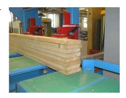
Is the cross section not square (e.g. beams not true to size, chamfers) it is possible that smaller indentation caused by the corrugation occur through the higher pressure on the surface. If necessary rotate the visible side of the work piece towards the fence. That is where the positioning wagons have an even surface and won't score the lumber.
