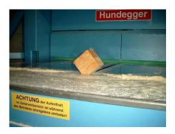
A change in tool geometry caused by sharpening has to be corrected in the machine data (d) with the required offset value.
