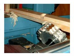
When processing work pieces with a small cross section there may be vibrations during processing which may lead to excessive tear out by the end mill due to the fact that the end mill is not chip limited. This could ultimately lead to the destruction of the work piece.
