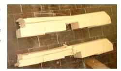
When processing profiled ends include an offset in the design. This pre-work will minimize tear out in the segment where the end mill will emerge. The picture on the right shows a large tear out which was caused by vibration and the missing offset in the design.
