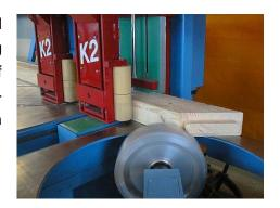
A big advantage of the milling head is the fact that the tool geometry does not change as the scoring knives always have the same measurement. Therefore, the milling head can be used to check other tools that may change their geometry by processing a complex work piece like a bird's mouth hip rafter. Is there a variance in height between the segments processed by the milling head and the end mill the machine data (d) has to
