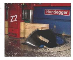
It has to be considered, that extremely short work pieces may need to be processed that be left on the saw table as the positioning wagon on the right hand side can't clamp it. Those pieces would end in the waste bin via the table opening.
