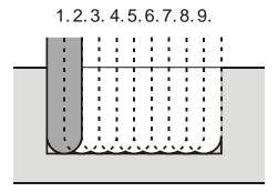
If a slot needs to be cut with a sword that is less wide than the slot the sword has to cut several times moving upwards until the programmed width is reached. A thin sword will bend during the second, higher cut and has a tendency to move toward the already processed area. Therefore, the width of the slot is smaller at the bottom than at the edge. This phenomenon can be avoided by selecting the proper sword. Another cause for the bending of the sword could be a knot in the wood.
