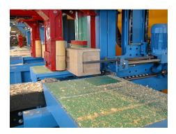
The so called "Wavecrest" which is caused by the round cutting shape at the bottom of the slot (drawing on the right) can be minimized by changing the setting in the machine data (d)  $\rightarrow$  operations  $\rightarrow$  overlap slot strokes  $\rightarrow$  Yes. This causes the work piece to be moved by half a cut width and results in an overall increased cutting depth. However, the processing takes longer (drawing below).
